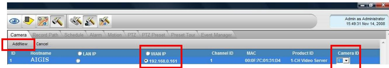
Figure 8.6 - Select Device, Assign ID
